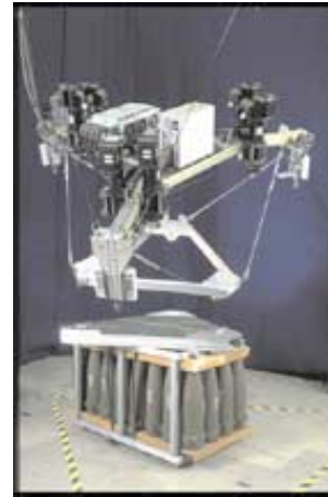
Fig. 3. RoboCrane for Material Handling at NIST, manipulating a payload. [4]
